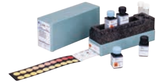
Chlorine dioxide measurement
