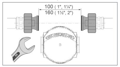
1. Install the water meter screw connections into the pipe (the installation dimension must be: 100 mm = for 1",  $1\frac{1}{4}$ " and 160 mm = for  $1\frac{1}{2}$ ", 2").
