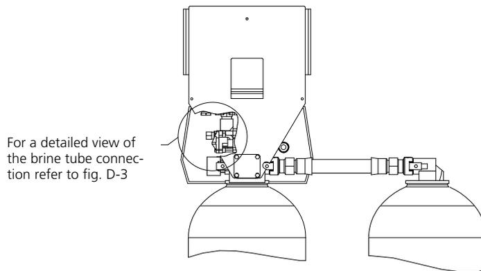
Fig. D-2: Water softener GENO-mat®-duo WE; rear view
