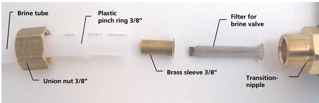
Fig. D-3: Exploded drawing of the brine tube connection
