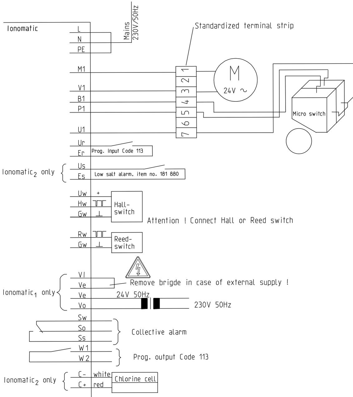
Fig. D-2: Terminal plan
