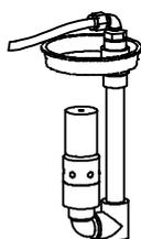
Brine valve with transition nipple and angle piece
