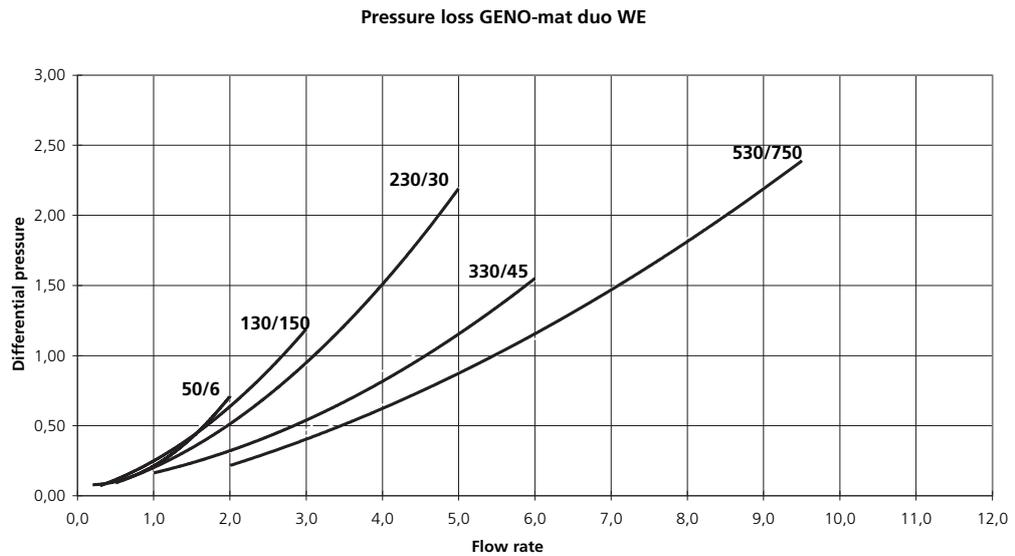
Fig. D-2: Pressure loss curve for GENO-mat® duo WE
