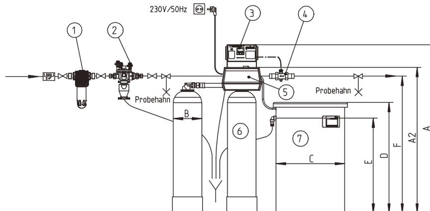
Fig. D-1 (a): Installation drawing for water softener GENO-mat®-duo WE
