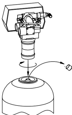
Remove the protective cap, fasten the control valve
