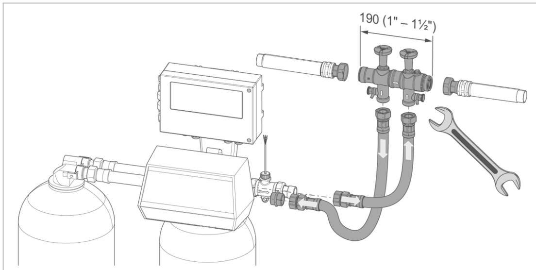
1. Install the screw connection into the pipe.
