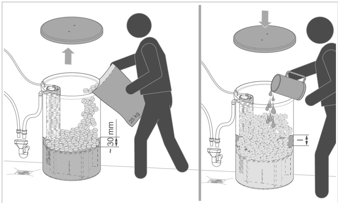
1. Remove the lid of the salt dissolving tank.
