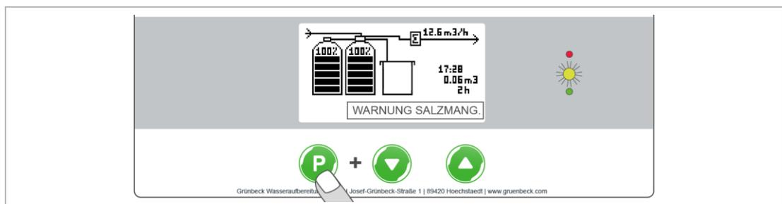
5. Acknowledge the warning **Low salt** on the control unit using the key **P**.
