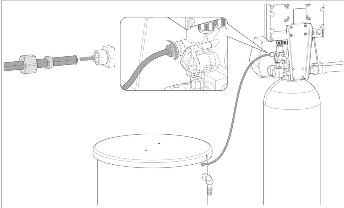
8. Fasten the brine hose on the injector with crimp ring, inserted support sleeve and union nut on the injector.
