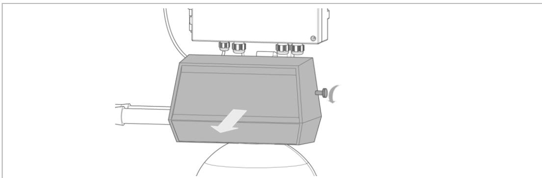
1. Unscrew the two knurled screws on the sides
