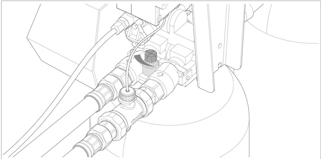
1. Open the on-site shut-off valve at the raw water inlet.
