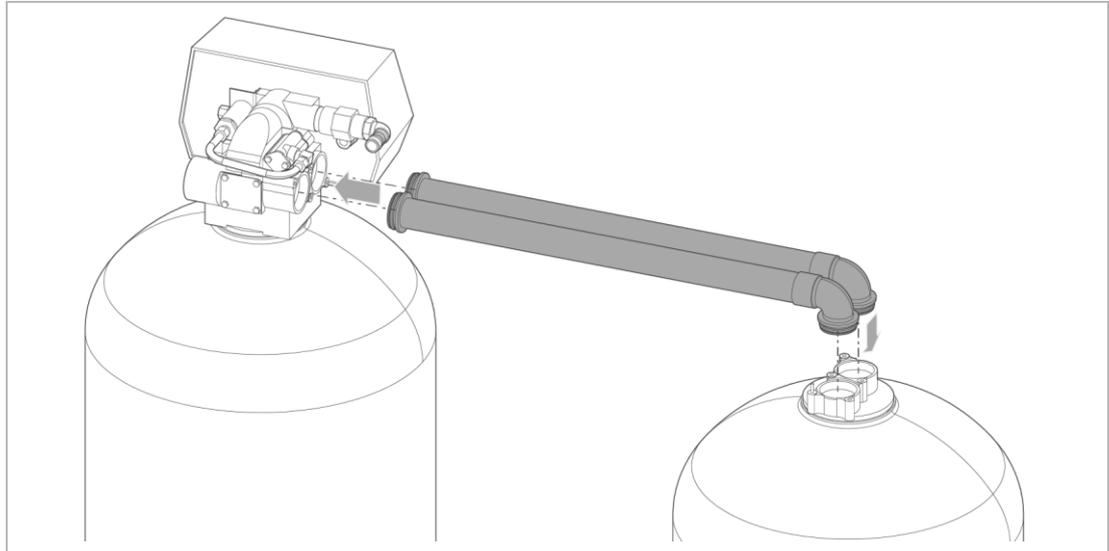
7. Install the connecting pipes between the control valve and the bottle adapter.
