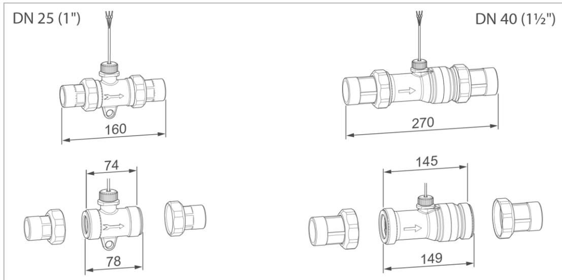
1. Prepare the soft water line for the installation of the water meter.
