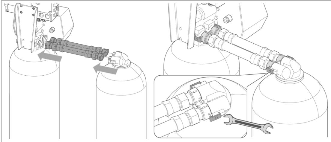
6. Install the connecting hoses between the control valve and the bottle adapter
