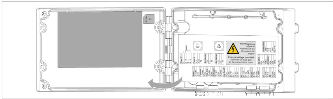
The SD card socket is integrated in the operating unit of the IONO-matic WE control unit.
