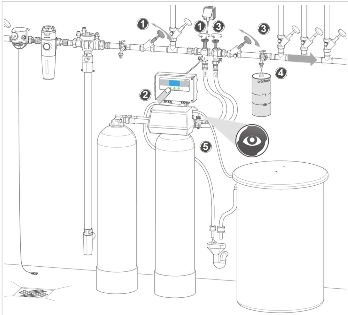
1. Open the shut-off valves on the raw water inlet.
